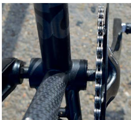
Above: The axle is unusually wide for a singlespeed road bike in order to make the chainline work with the 135mm threaded hub. That means a wider pedal tread, which some won't like and others won't mind
