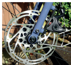
Top: Bottom gear is 26/36, which is fine for loaded touring Bottom: Tektro Spyre-C cable discs provide reliable braking
